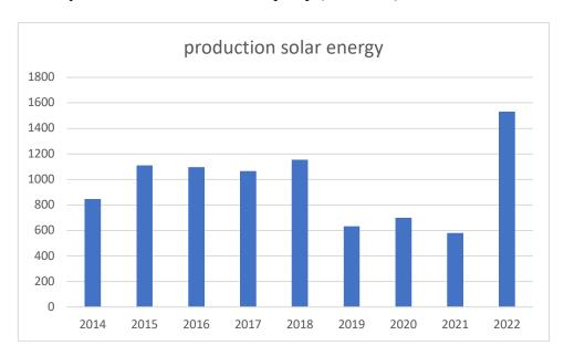
Solar thermal energy is obtained via 4.6 m2 of solar panels that heat a 300 l solar water tank (next to guest room Tilia). Backup is provided by an air/water heat pump and on top of that by the fuel oil boiler. The production reduction in 2019 is mainly related to increasing the boiler temperature from 55°C to 63°C due to comfort demand from our guests ...: filling a second bathtub.
